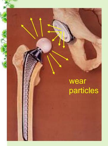
Wear particles from the replacement head and liner cause inflammation that can lead to pain, bone loss, and ultimately revision surgery
