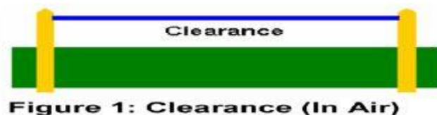
Figure 1: Clearance (In Air)
