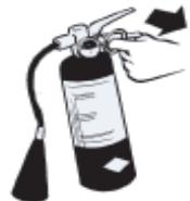
**P**ull the pin at the top of the extinguisher.
