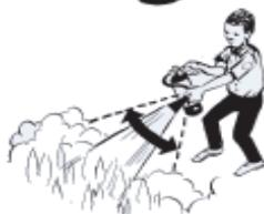
**S**wEEP the nozzle back and forth at the base of the fire.
